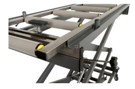
Coffin carrier roller device - Equipment specially designed to be adaptable to our range of trolleys with rails for body trays on wheels. It makes it possible to transfer coffins with bottom flat on roller conveyor. A set of five PVC rollers fixed on a 304 L stainless steel frame between the rails of the trolley allows easy conveyance. There is a coffin locking system included – operated manually.
